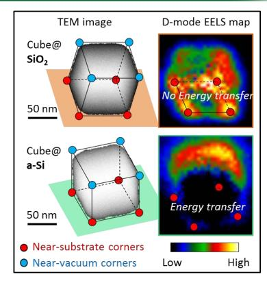
Mapping energy transfer in Ag nanocube@substrate systems: The EELS map of the dipole (D) mode in the cube@SiO<sub>2</sub> system shows strong substrate-localization, indicating that no energy transfer occurs at the interface. In contrast, the near-zero EELS signal at the cube@a-Si interface is the signature of energy transfer.
