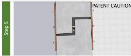
Threaded bars are placed
