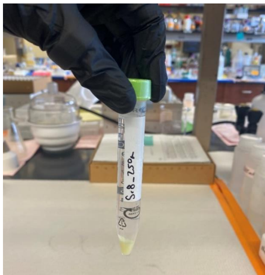
Figure 4: Strontium (pH 8, 250 ppm U_{60} ) reaction after two weeks of equilibration. It is visually apparent that separation has occurred due to the distinction between clear solution and solid.
